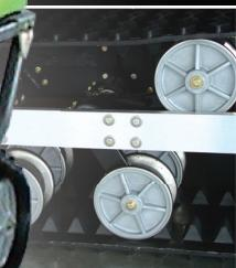
Added additional front axle with torsion suspension and upper idler assembly.
